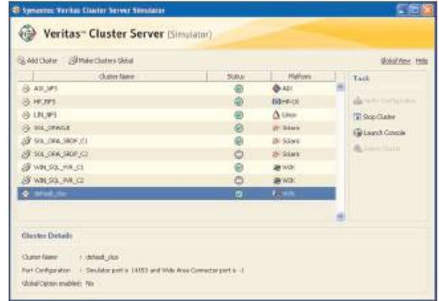
Figure 3. By using Veritas Cluster Server Simulator, administrators can ensure that critical applications are running on an optimal set of servers in the cluster configuration.
